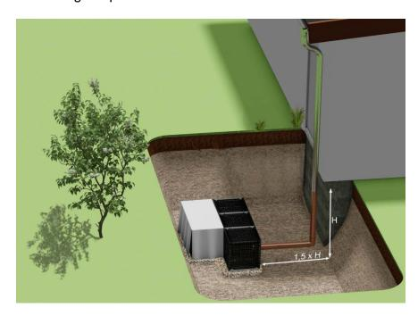
The percolation system should always be planned and installed near the rainwater connection. The distance to buildings should be 1.5 x the height of the basement/foundation, whereby the pit depth depends on the planned height of the rainwater connection. Ensure sufficient distance to trees, especially to their roots (tree crown diameter = distance to the percolation system).
